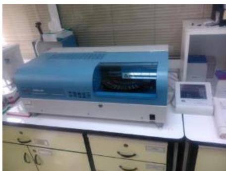
*Figure 3.6 - DMA 80 Mercury Analyzer*
