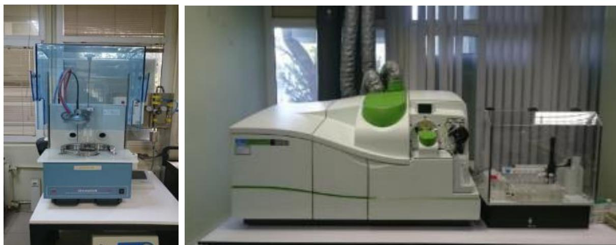
*Figure 3.5 - ICP-MS instrument and microwave combustion system*
